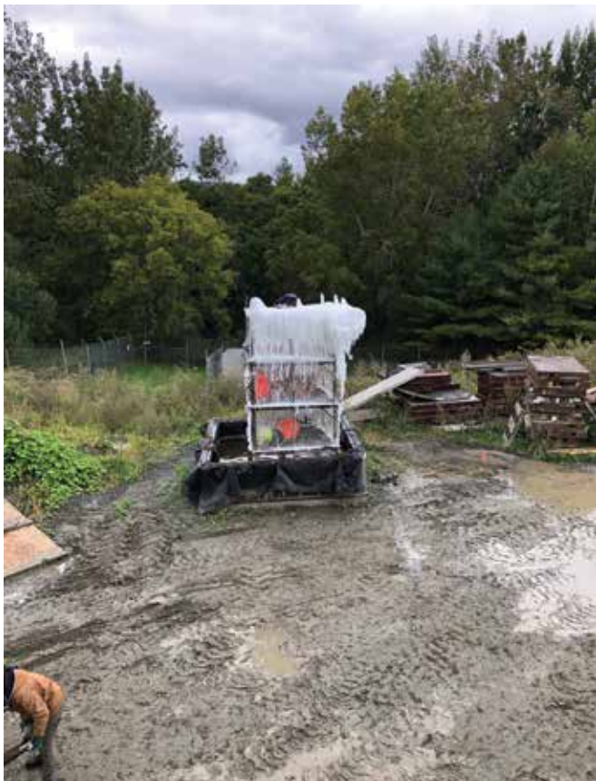
Ice accretion as viewed from 45 ft., part of the tests carried out at CRREL's facilities. Photo courtesy M. J. Lewandowski
