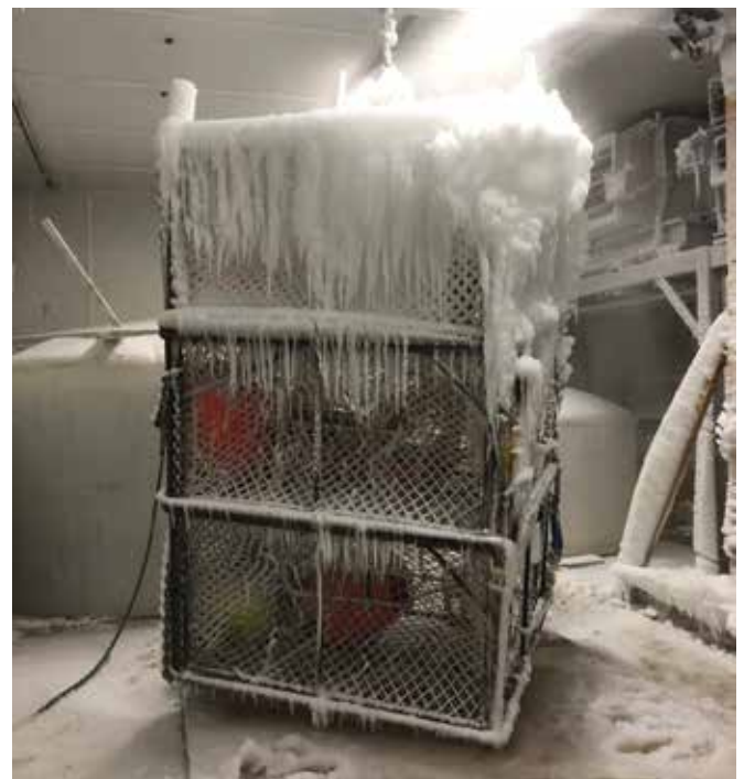
The materiel evaluation facility test chamber at CRREL in Hanover, NH, showing a 3-pot stack and oscillating spray nozzle. Photo courtesy M. J. Lewandowski.
